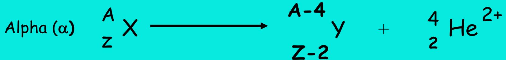
With an alpha particle 2 protons + 2 neutrons are emitted
