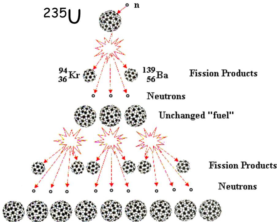
In nuclear fission the nuclei of heavier elements break up into two smaller lighter nuclei and release a large output of energy.  $^{239}\text{Pu}$  and  $^{235}\text{U}$  are the only important fissionable isotopes. 0.7% of natural uranium contains  $^{235}\text{U}$ . enrichment of uranium ore produces 2-3%  $^{235}\text{U}$ , sufficient for fission.
