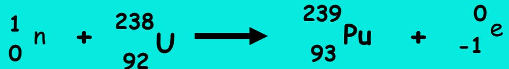
**Plutonium** does not occur naturally but is capable of fission and is therefore used as an alternative fuel. Fast travelling neutrons are needed, so a moderator is not needed.
