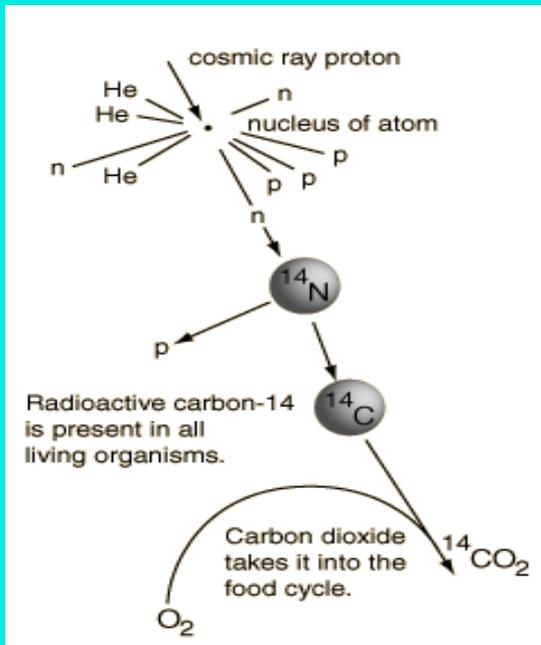
Measurement of the beta decay activity of a buried piece of wood provides a measurement of the time elapsed since it was living and in equilibrium with the atmosphere.
